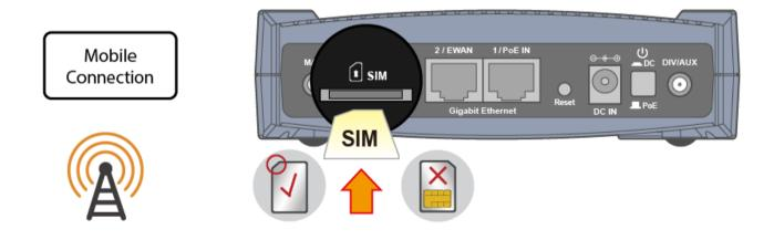
WARNING: Please power off the device before inserting or removing the SIM
